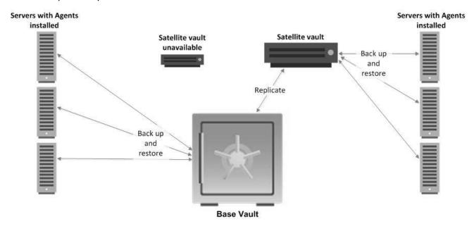
For N:1 replication, you must use customer license quotas to limit the amount of storage or number of Agents and plug-ins that a specific customer can use. When you create customers, locations, accounts and users on the Base vault, they are replicated on the Satellite vaults.
