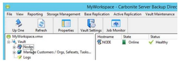
To determine which services are running, point to the node's Status column.
