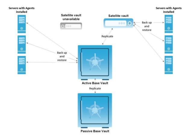
As shown in the following diagram, if the Active Base vault fails, you can fail over from the Active Base vault to the formerly Passive Base vault. Data from the Satellite vaults is then replicated directly from the Satellite vaults to the new Active Base vault.
