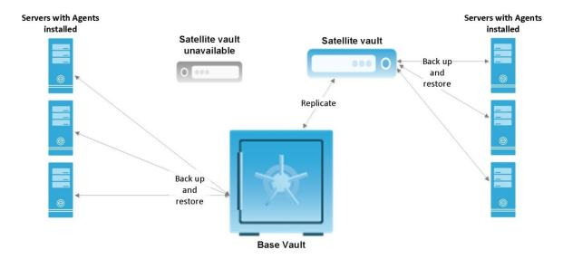
For N:1 replication, you must use customer license quotas to limit the amount of storage or number of Agents and plug-ins that a specific customer can use. When you create customers, locations, accounts and users on the Base vault, they are replicated on the Satellite vaults.
