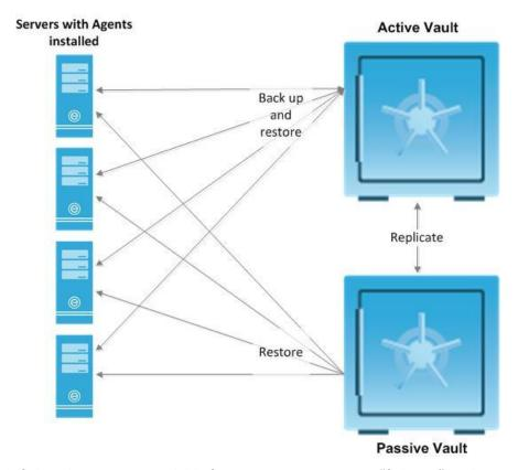
If the Active vault fails or becomes unavailable for some reason, you can "fail over" to the Passive vault so that the formerly Passive vault becomes the new Active vault. Failover does not happen automatically; you must manually fail over to the Passive vault. As shown in the following diagram, Agents then bypass the formerly Active vault, send backups directly to the formerly Passive vault, and restore data from the formerly Passive vault.
