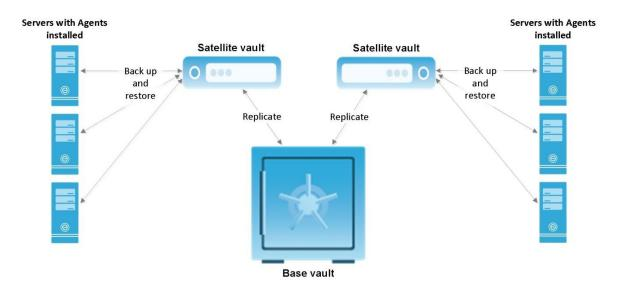
As shown in the following diagram, if a Satellite vault fails or becomes unavailable for any reason, Agents send backups directly to the Base vault and restore data from the Base vault.
