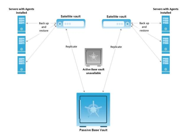
When the previously Active Base vault becomes available again, you must run replication from the current Active Base vault to synchronize the data. After synchronization, you can leave the vault assignments as they are, or change the current Passive Base vault into the Active Base vault again. If you change a Passive Base vault into an Active Base vault without synchronizing and replicating the data, all unreplicated data is permanently deleted.
