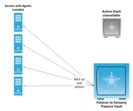
In 1:1 replication, safesets are replicated if they are online and unexpired. Data stored in archives and secondary storage pools are not replicated. Safesets on the Active vault can be replicated to the Passive vault when a backup completes successfully, or you can schedule them to replicate on specific days at a specific time.
