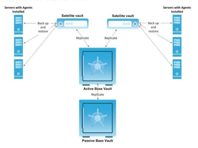
As shown in the following diagram, if a Satellite vault fails or becomes unavailable for some reason, Agents can send backups directly to the Active Base vault, and data can be restored from the Active Base vault.
