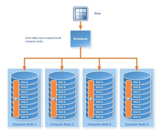
The above diagram depicts how a row would be stored within a replicated table. A replicated table is striped across all of the disks assigned to each of the distributions within a compute node.
