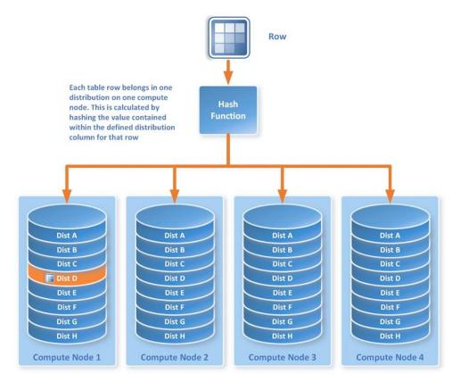
Each SQL Server PDW compute node has eight distributions and each distribution is stored on its own set of disks, therefore ring-fencing the I/O resources.
