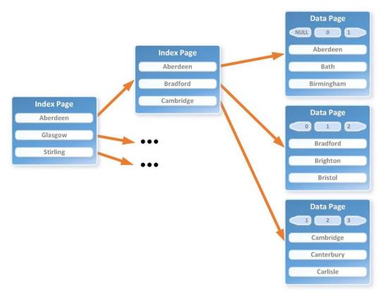
When defining a clustered index on a distributed table within PDW it is not necessary to include the distribution column within the cluster key. The distribution column can be defined to optimize the joins while the clustered index can be defined based upon the most frequently used columns as predicates or range operations.
